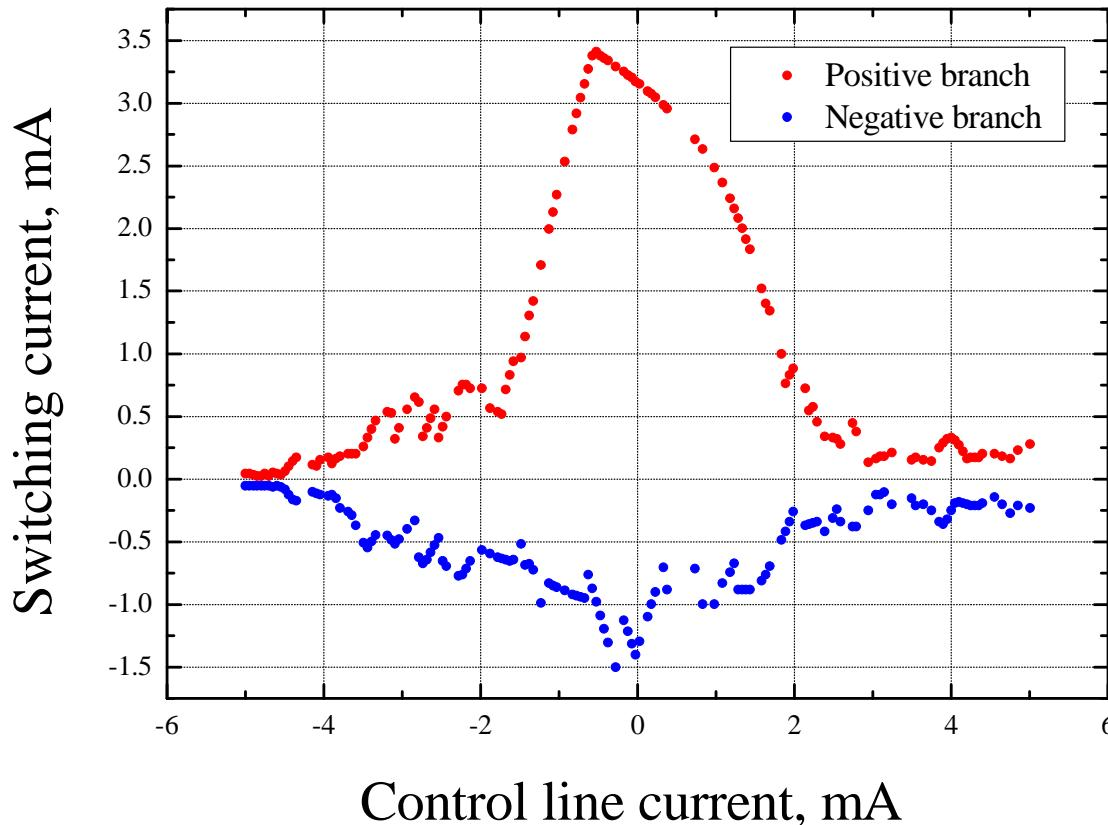
Strong perpendicular magnetic field influence observed (no cryo-permalloy shield was used, due to the He-3 cryostat restrictions ).
